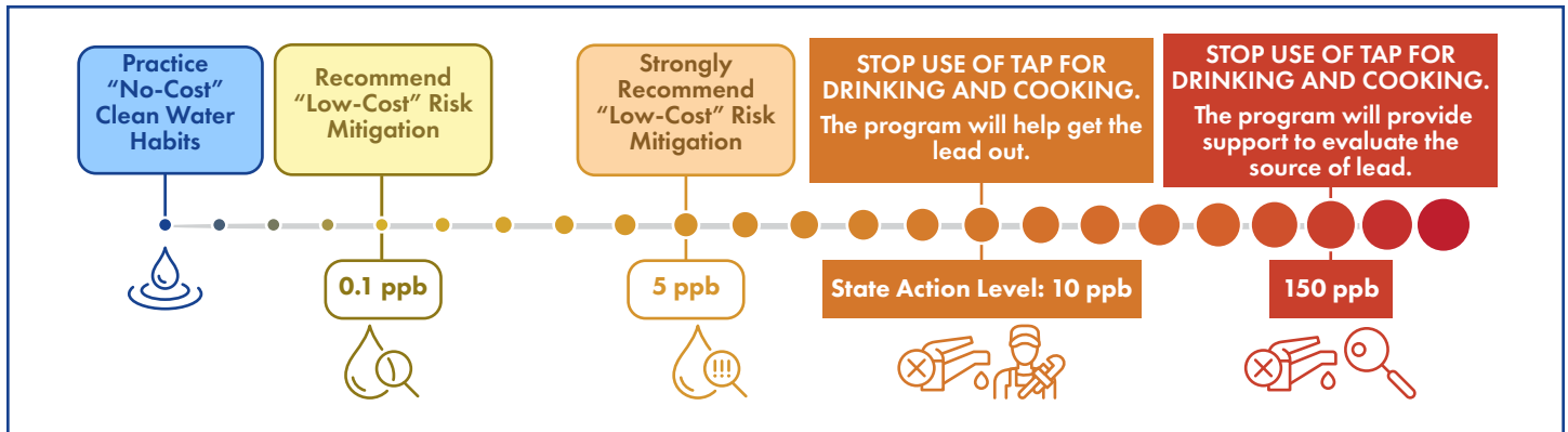
Figure 2. Illustration of Recommended Risk Mitigation Based on Test Results for Each Tap.
